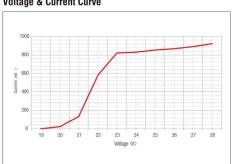
Note: This curve is tested when the IP20 1M LED Strip is under thermal stability after 2hrs continuous working in 15 °C room temperature.
