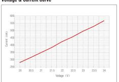
Note: This curve is tested when the IP20 1M LED Strip is under thermal stability after 2h continuous working in 15 °C room temperature.
