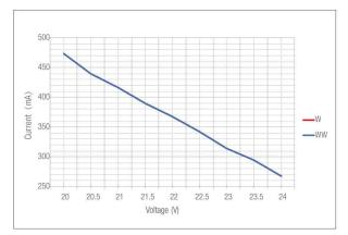
Note: This curve is tested when the IP20 1M LED Strip is under thermal stability after 2h continuous working in 15 °C room temperature.
