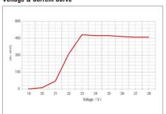
Note: This curve is tested when the IP20 1M LED Strip is under thermal stability after 2hrs continuous working in 15 °C room temperature.
